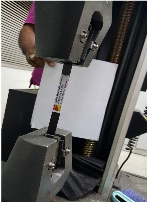
Testing Equipment, Method of Tester Installed, Once Tested the CFRP Cured Laminates Breaking
